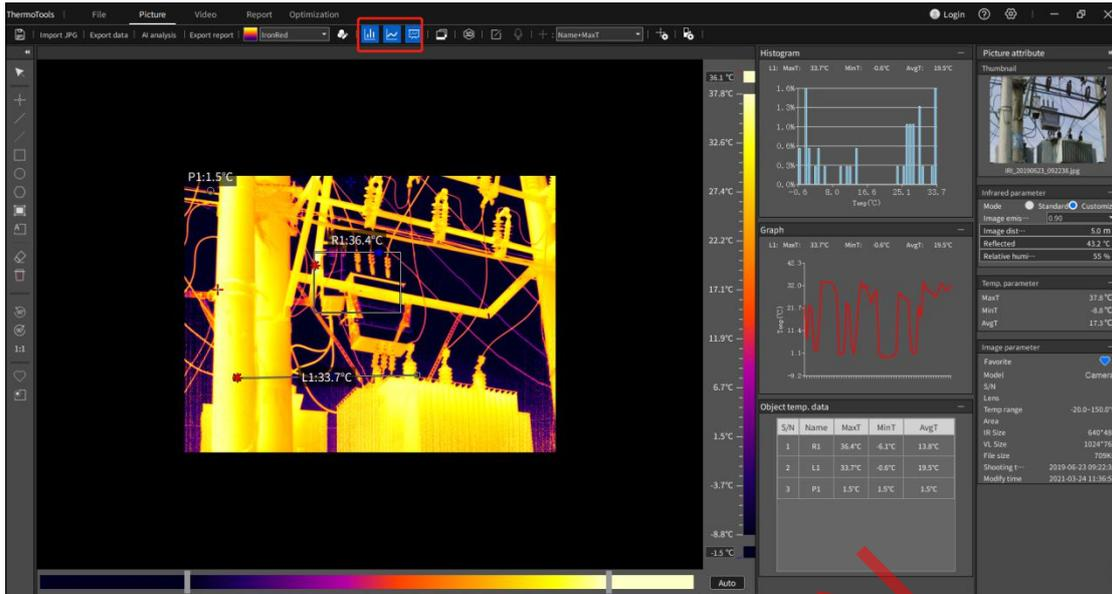
Figure 3-12 Histogram, Line Chart and Object Data
