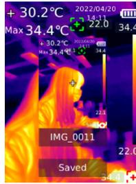
Press the trigger to capture an image. Press the Left/Right button to save it or not, and press the SET button to confirm or the Return button to cancel. In the auto save mode, the images will be automatically saved to the SD card.
