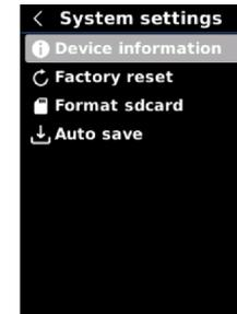
In the Settings interface, press the Up/Down button to select "System settings", and press the SET button to enter its setting interface. Press the Up/Down button to select Device information/Factory reset/Format SD card/Auto save, and press the SET button to enter the submenu. Press the Return button to return to the previous interface.
