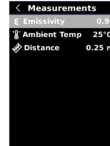
In the Settings interface, press the Up/Down button to select "Measurements", and press the SET button to enter its setting interface. Press the Up/Down button to select Emissivity /Ambient temp/Distance, and press the SET button to set the selected parameter. Press the Up/Down button to add/subtract the value, and press the SET button to confirm. Press the Return button to return to the previous interface.
