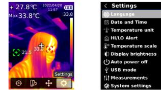
In the main interface, press the SET button to open the main menu. Press the Left/ Right button to select "Settings", and press the SET button to open its submenu. Press the Up/ Down button to select an option in the submenu, and press the SET button to enter its setting interface. Press the Return button to return to the previous interface.
