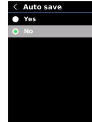
In the system settings interface, press the Up/Down button to select "Auto save", and press the SET button to enter its submenu. Press the Up/Down button to select Yes/No, and press the SET button to confirm. Press the Return button to return to the previous interface.
