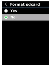
In the system settings interface, press the Up/Down button to select "Format SD card", and press the SET button to enter its submenu. Press the Up/Down button to select Yes/No, and press the SET button to confirm. Press the Return button to return to the previous interface.
