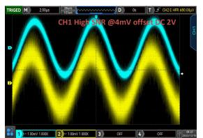
Set small signal superimposed large DC, UTG1000X output noise is lower, with higher SNR.
