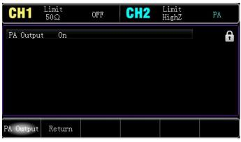
The power amplifier (on -PA model only) can boost the out to a maximum of 4 W, up to 100 kHz with a slew rate greater than 18 V/µs
