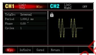
Supports pulse string mode: "N cycle", "Gating", "Infinite" Two modulation signal sources: "Internal" and "External".
