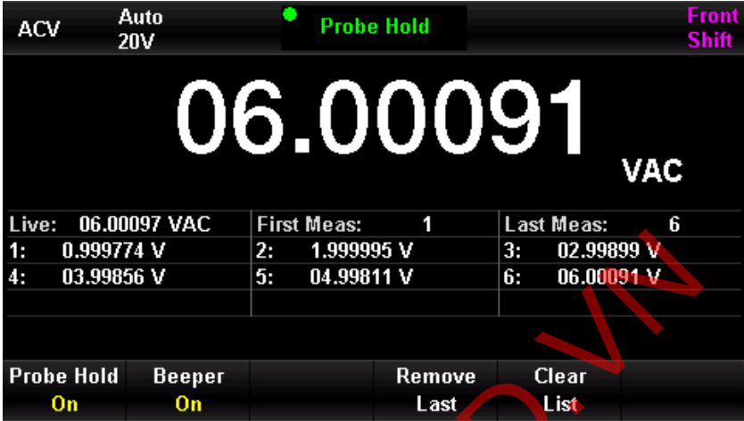
Figure 4-11 ACV Hold Measurement Menu
