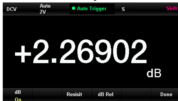
Figure 2-45 Interface of dB operation
