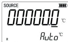
Picture 3.2-1 Auto cold junction temperature compensation
