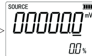
Picture 1.1-6 Voltage output 1000mV
