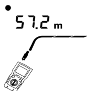
Figure 6.15 Open on Coaxial Cabling
