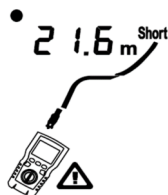
Figure 6.16 Short on Coaxial Cabling
