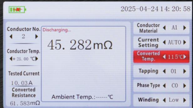
Two preset conversion temperatures (75°C and 115°C) are available to accommodate diverse testing scenarios.
