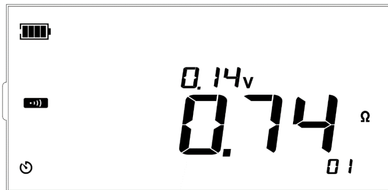
Figure 13.16 Test leads are shorted
