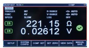
Can set the impedance and voltage upper and lower limit comparison function
