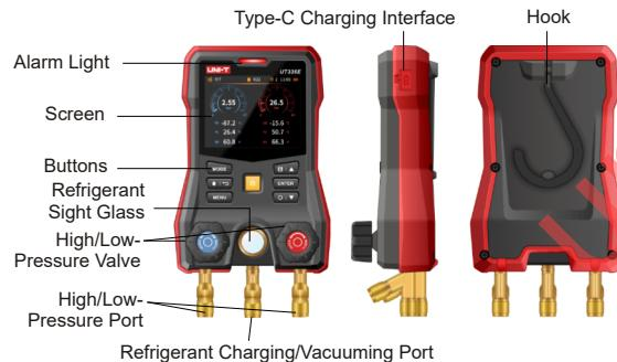
High/Low-Pressure Port: 1/4 SAE refrigerant hose connection; connect a blue hose to the left-side port (low-pressure port); connect a red hose to the right-side port (high-pressure port).
