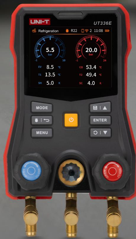
The UT336E KIT facilitates the installation, debugging, and maintenance of refrigeration and heat pump systems. It accurately measures high and low-side pressures and, when paired with two wireless temperature clamps, calculates superheat and subcooling to optimize performance. The device includes built-in refrigerant parameters and enables remote monitoring via a wireless app.
