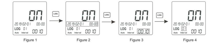
d) After setting the parameters, press the SET button or pull the trigger to return to the HOLD interface. The Auto Interval icon will flash. When the start time of the scheduled measurement is reached, the thermometer will automatically start temperature measurement and store the current time and measured value. Each time the interval time is reached, the thermometer will automatically measure and store the current data, until the last interval.
