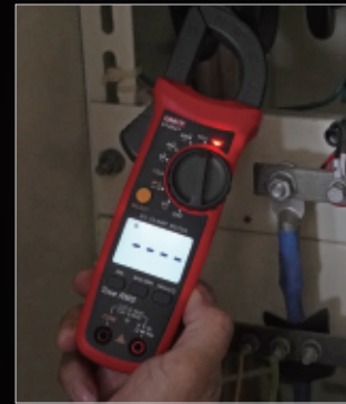
NCV multi-segment display and audio/visual alarm
