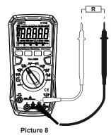
Insert the red test lead into the <sup>→ 1(-Hz</sup> <sub>V Ω→)</sub> or <sup>→ 1(-Hz</sup> <sub>V Ω→)</sub> c terminal, and black test lead into the COM terminal.
