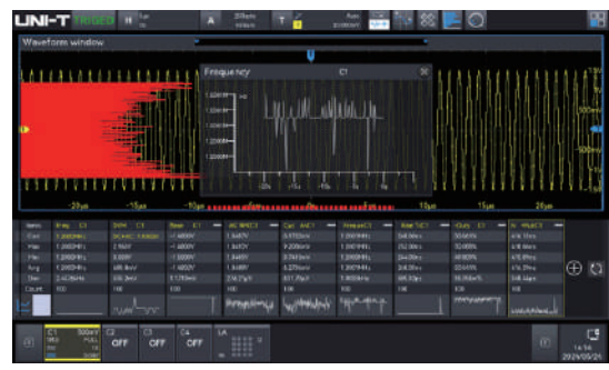
● MSO3000X series provides 54 kinds of measurement parameters. The parameter snapshot displays 39 kinds of test items for a single channel measurement
