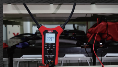
DC current test of Battery modules
