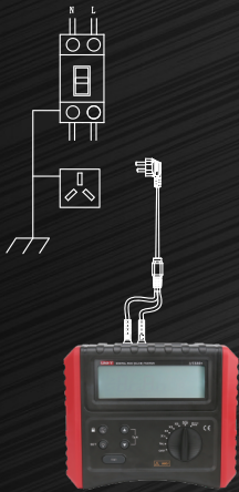
single phase socket RCD test
