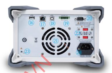
①LCD display ②Function key ③Digital keyboard ④Rotary encoder ⑤Shift key ⑥Channel selection and output control ⑦Keyboard lock ⑧Preset key ⑨System settings ⑩Home key ⑪CH3 quick selection ⑫Operation menu ⑬Power switch ⑭CH4 output ⑤Output channel and indicator ⑥USB HOST ⑰LAN ⑧USB device ⑨Digital IO ②RS232 ㉑Fan ②Input source selection ㉓Protected GND ②AC socket
